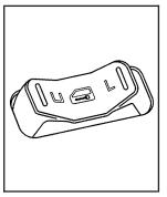
The power door lock switches are located on the driver's and the front passenger's armrests.
